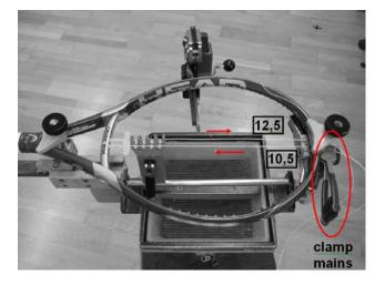
Figure 3 Install left side mains
